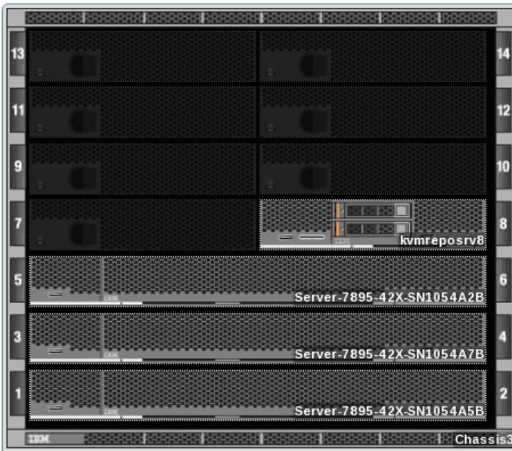
Figure 2. The destination server for LPM occupies slots 1 and 2 in Chassis 3
