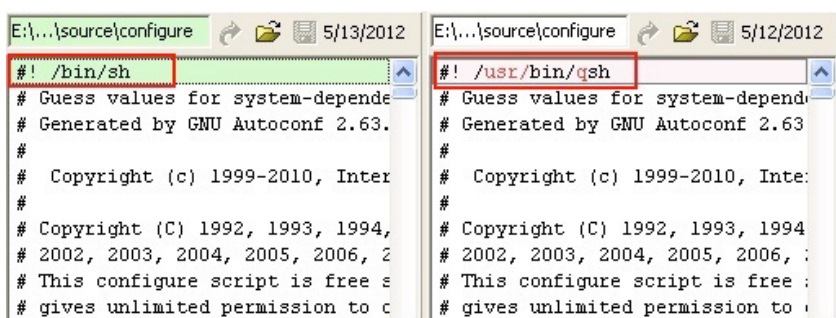
Figure 20. Header of the two different configuration files
