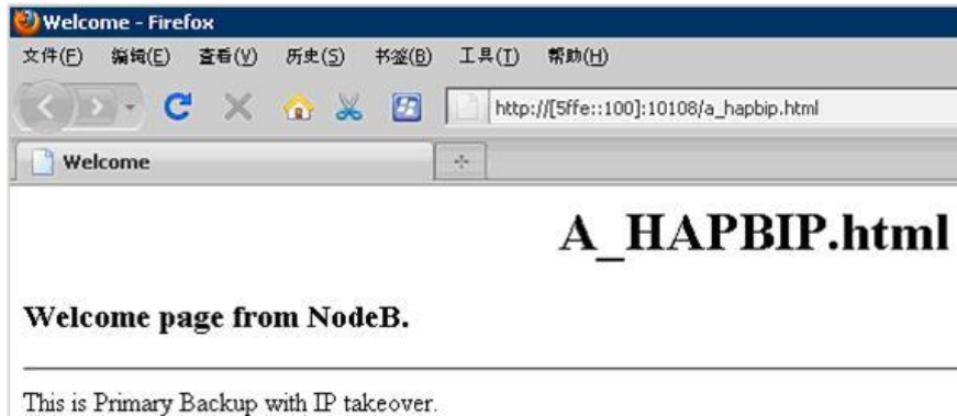
Figure 8. Primary or backup with IP takeover - Backup server on NodeB is up and running
