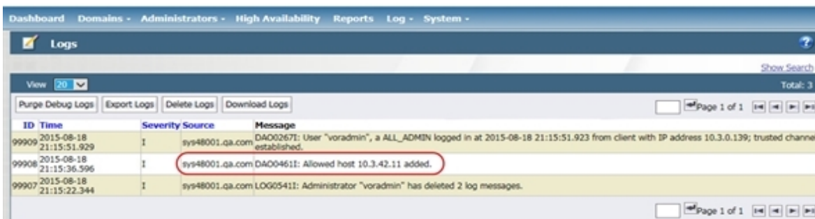
Figure 11-3: Log entry indicating an SNMP server has been added to the ACL
