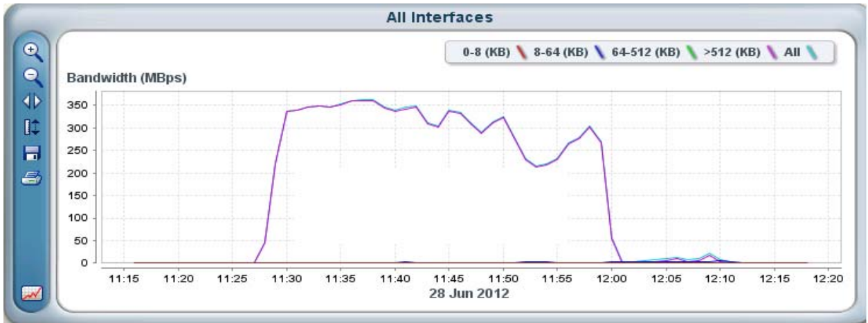
Figure 4: SAS I/O characteristics with 40 session benchmark workload (most of the I/O is 512 KB and above)
