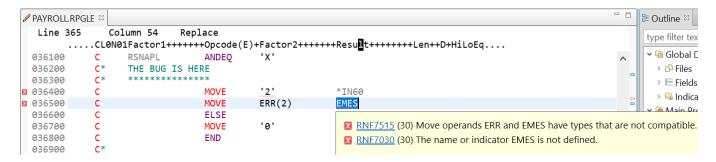
The variable EMES should be EMESS. One good way of finding the correct name is the content-assist tool.
