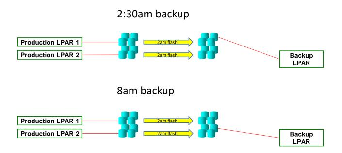
The controlling LPAR can manage the host connections of the Backup LPAR to its disks. This allows one backup LPAR to sequentially service the backups of multiple production LPARs, reducing the footprint of the total solution.
