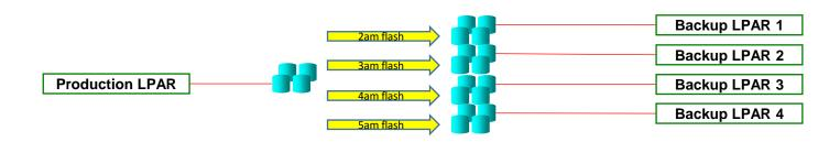
When one production LPAR hosts multiple applications which quiesce at different times, or an application that has both pre-batch and post-batch processing, our toolkit can manage concurrent flashcopy operations. In these scenarios each backup LPAR typically backup only a portion of the data, i.e. the data associated with a specific application. Note that a quiesce or memory flush affects the entire production LPAR, not just one application.
