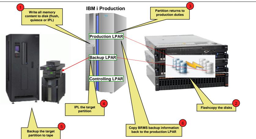
Controlling LPAR with IP connection to production/backup LPARs, HMC and external storage is key to manage the Full System FlashCopy process as FlashCopy cannot be invoked from a quiesced or powered off production LPAR
