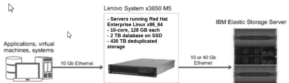
Figure 4. Logical layout for a medium IBM Elastic Storage Server system
