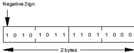
Figure 101. Integer Representation of the Number -21544
