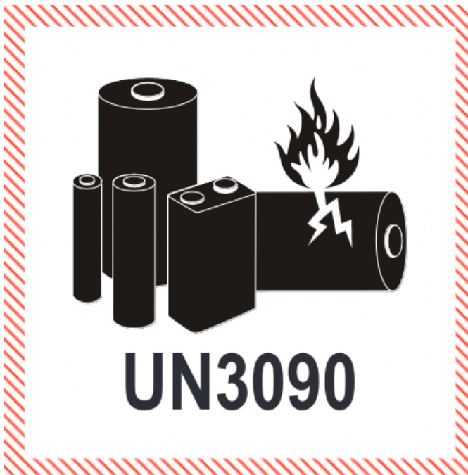
Figure 3 - Example below of a Lithium Metal Battery Mark (UN3090) IBM PN 03FN645
