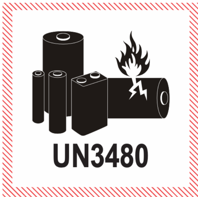
Figure 1 - Example below of a Lithium Ion Battery Mark (UN3480) IBM PN 03FN643
