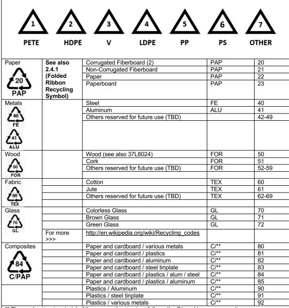
\*\* The predominant material of the composite structure follows the C/ marking on composites
