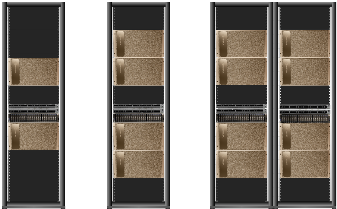
Figure 14: Two, four, and eight DGX A100 system configurations
