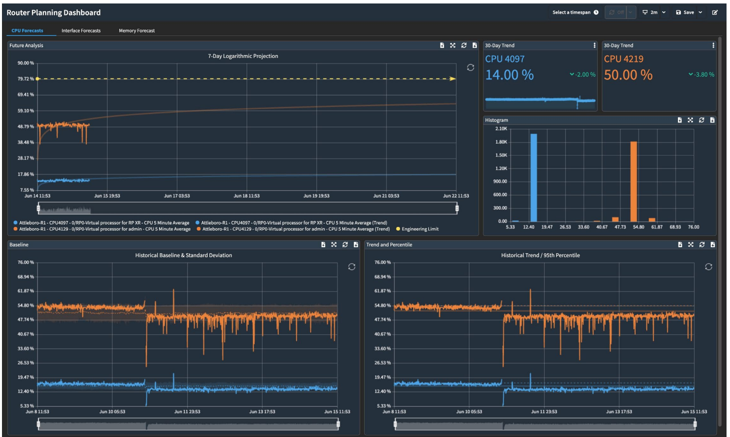
Figure 2. Capacity planning reports can help you forecast expected resource utilization and exhaustion.
