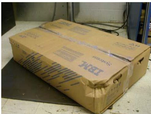
Packaging Condition After Drop Testing (10 drops from 76 cm)
