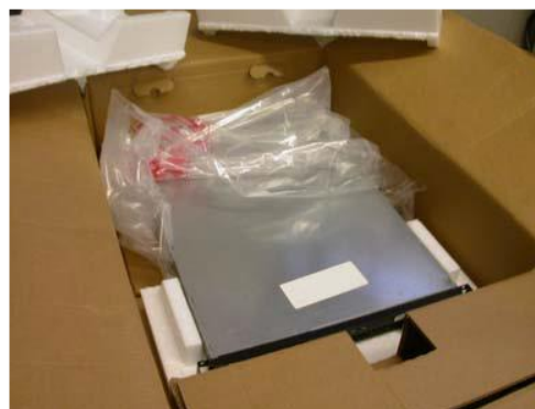
Packaged Product After Drop Testing (Result: Pass. No physical or functional defects)
