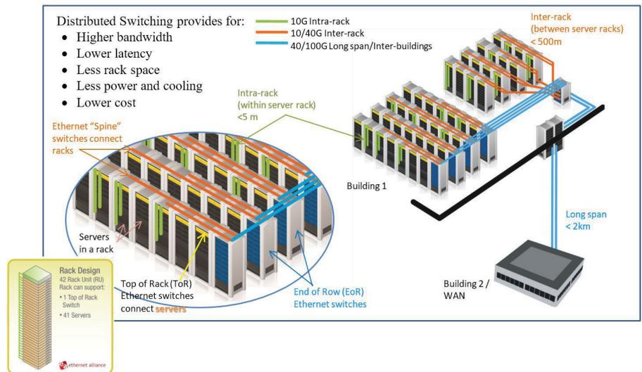
**Figure 3:** Illustration showing data center connections. The shorter server-to-server connections within the server rack typically require <5m (green) of routing, longer connections between the server racks may require up to 500m (orange), and long span connections within a building or between buildings can measure up to 2km (blue). SOURCE: Image courtesy of Finisar, Patterson Group, IBM, Ethernet Alliance
