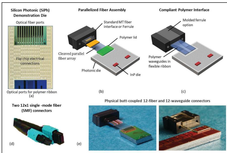
**Figure 7:** a) IBM silicon photonic die; b) schematic representations of the parallelized fiber and c) compliant polymer ribbon assemblies; d) an industry standard 12x1 single-mode fiber connector; e) photos of the parallelized fiber and compliant polymer structures. SOURCE: Images courtesy of IBM Corporation
