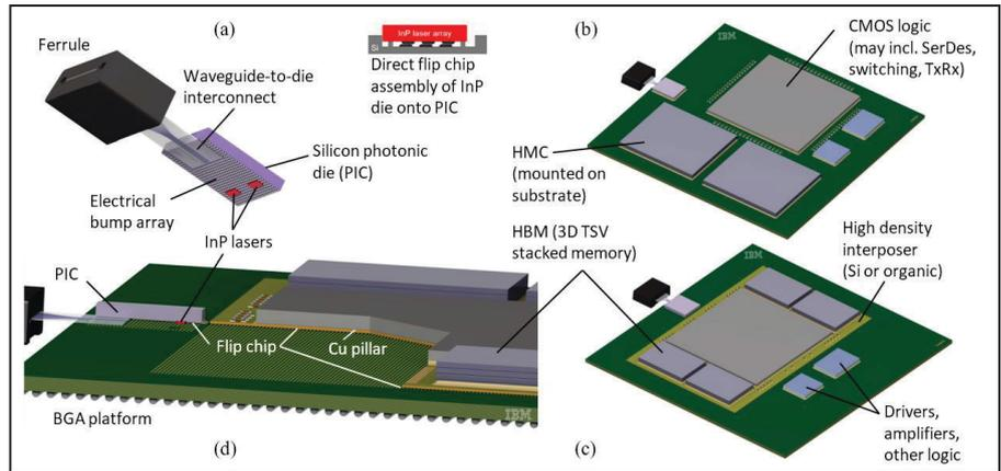
**Figure 4:** Silicon photonic MCM illustrating (clockwise) a) a photonic integrated circuit (PIC) with flip-chip mounted laser die and edge-coupled waveguide; b) logic, HMC and PIC mounted directly to a BGA substrate; c) logic and HBM mounted on a high-density interposer with copper pillar micro-bumps that enable high-speed connectivity; d) cut-away revealing copper pillar, flip-chip, BGA and optoelectronic interconnections. SOURCE: Image courtesy of IBM Corporation
