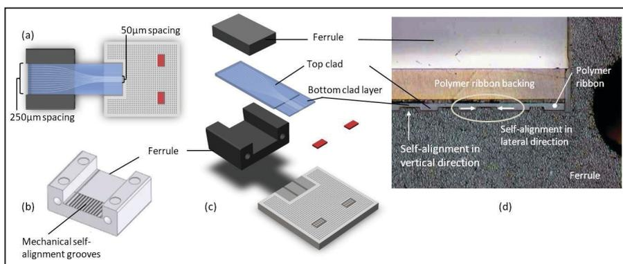
**Figure 9:** a) Top down view of compliant polymer ribbon aligned with ferrule (no lid) and silicon photonic die; b) ferrule with self-alignment guides for polymer ribbon; c) exploded view of assembly showing two-piece molded ferrule; d) cross section of polymer ribbon aligned to grooves in the molded ferrule. SOURCE: Images courtesy of IBM Corporation
