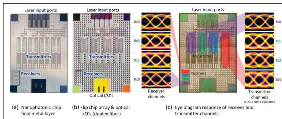
**Figure 5:** An IBM silicon (nanophotonic) wavelength division multiplexed 4 x 25Gb/s reference design (die) supporting both electrical and optical circuits. Two optical I/Os are seen at the bottom of the die. These connect to optical fibers, one in and one out. SOURCE: Images courtesy of IBM Corporation
