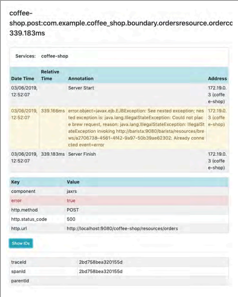
Figure 5-7. Zipkin trace details for a failed ordercoffee request
