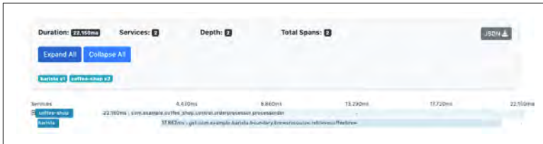
Figure 5-8. Zipkin trace for an application-defined span for processorder
