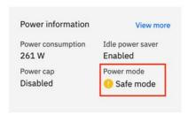
To re-enable full EnergyScale functionality, a reboot, firmware update, FRU replacement, or complete A/C power cycle of the system must be completed. If the problem which originally caused the system to enter safe mode is still present, the system will re-enter safe mode and generate an additional error log entry.
