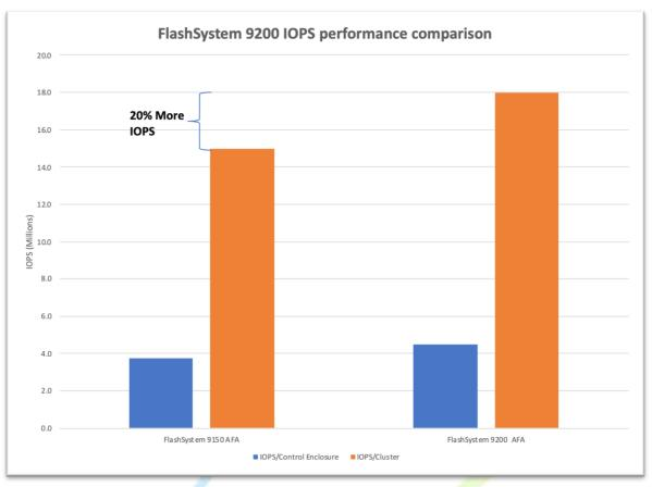
The new FlashSystem 9200/9200R AFA offers up to 20% more IOPS at 4.5M IOPS per control enclosure or 18M IOPS per cluster, along with 20% more bandwidth at 45 GB per sec per control enclosure or 180 GB per sec per cluster, than the priorgeneration (FlashSystem 9150) system.
