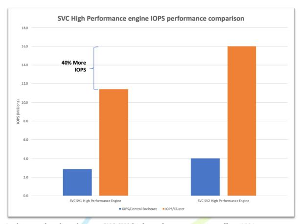
As discussed earlier, the new SVC SV2 high-performance engine offers 40% more IOPS than the previous-generation SVC SV1 high-performance engine at the same price. It offers up to 4M IOPS per control enclosure, or 16M IOPS per cluster with up to 48.8 GB per sec per control enclosure or 195 GB per sec per cluster of data bandwidth.
