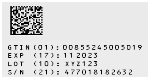
Figure 2: The pharmaceutical pack is marked with a barcode encoded with the serial number (AI: 01), Global Trade Item Number (GTIN, AI: 21), lot (AI: 10) and expiry date (AI: 17).
