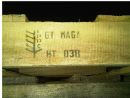
Figure 4 1 – Mark does not contain the required borders.
