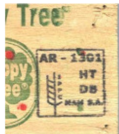
Figure 5 1 – Orientation of information does not match the examples in Annex 2 of ISPM 15:2009. Information included within the borders of the mark exceeds the requirements.
