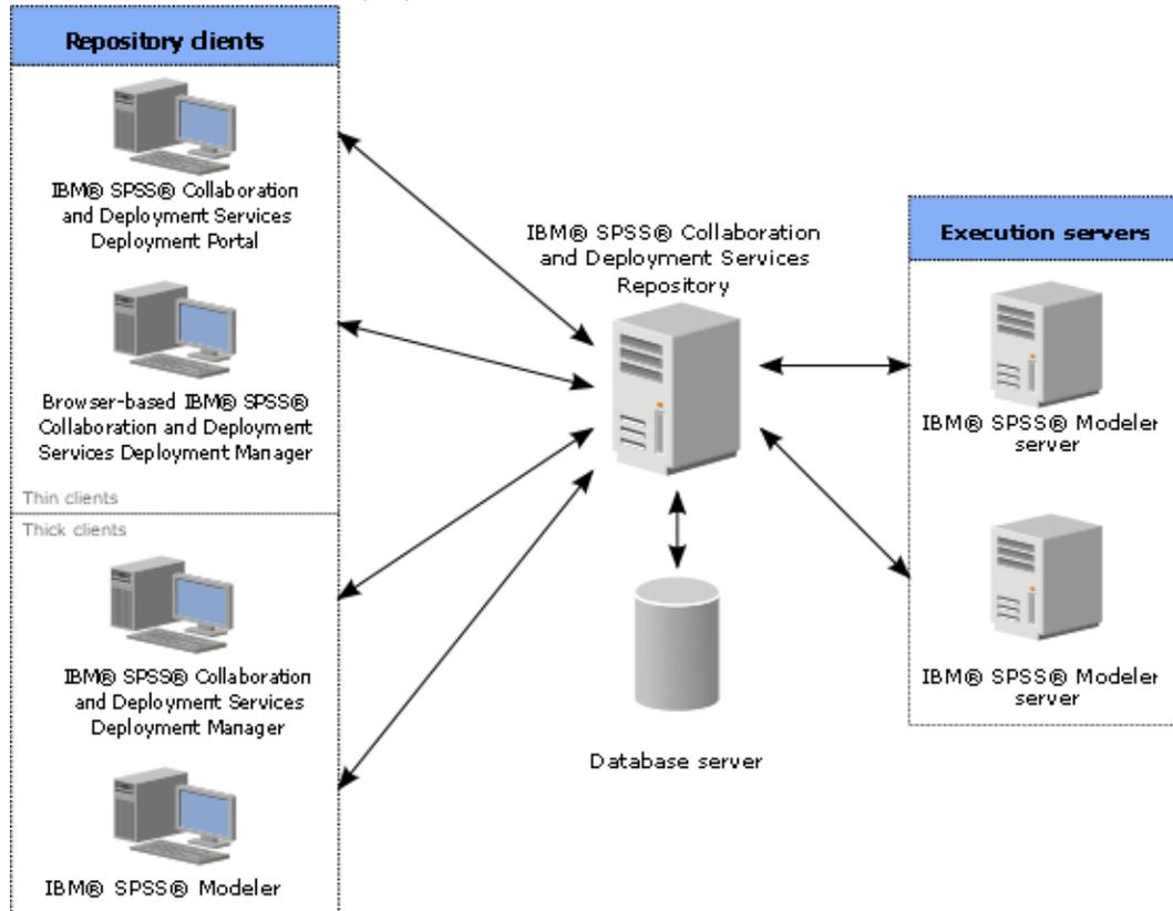
圖 1: IBM SPSS Collaboration and Deployment Services 架構
