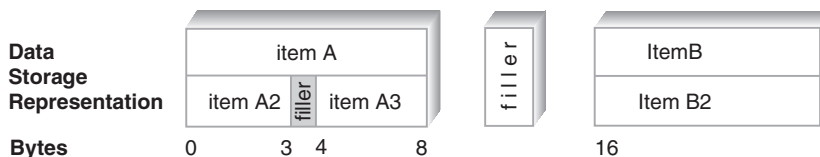
Figure 11. Data Storage Representation Without and With Synchronization
