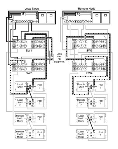
Sample diagram of Brocade 5000 32port cabling for virtual channels
