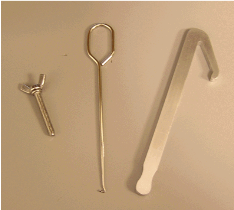
Figure 8. Rail tools, from left to right; UPG rail removal bolt tool, UPG rail removal puller tool, and Vertiv rail removal tool.
