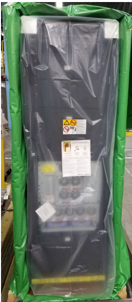
Figure 4. Frame packaged in clear white poly bag and green vapor barrier bag
