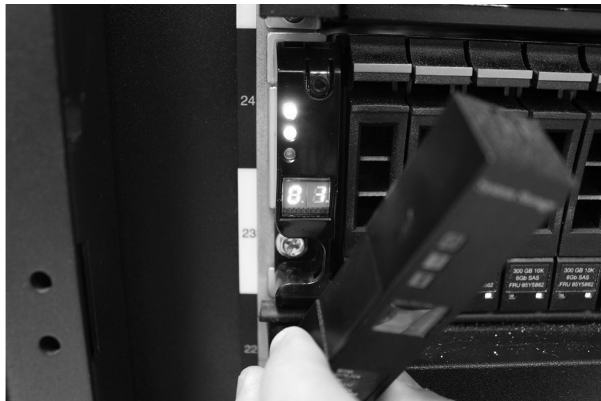
Figure 6. Removing the enclosure end cap
