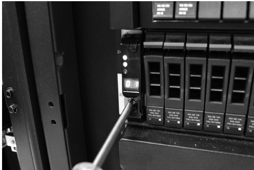
Figure 7. Securing an enclosure to a rack cabinet
