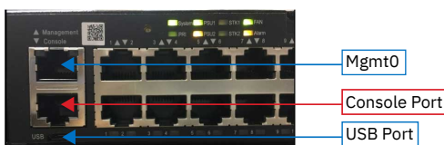
Figure 24. Switch port and switch markings
