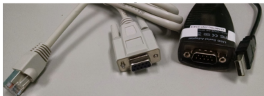
Figure 25. RJ45 to serial cable and USB to serial cable
