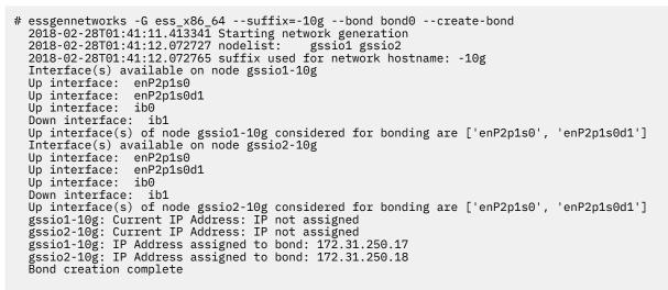
3. This example shows running **essgennetworks** to obtain information of high-speed interfaces IP address assigned to the bond for InfiniBand interfaces.
