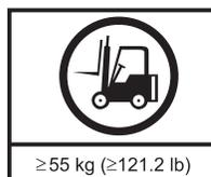
The weight of this part or unit is more than 55 kg (121.2 lb). It takes specially trained persons, a lifting device, or both to safely lift this part or unit. (C011)
