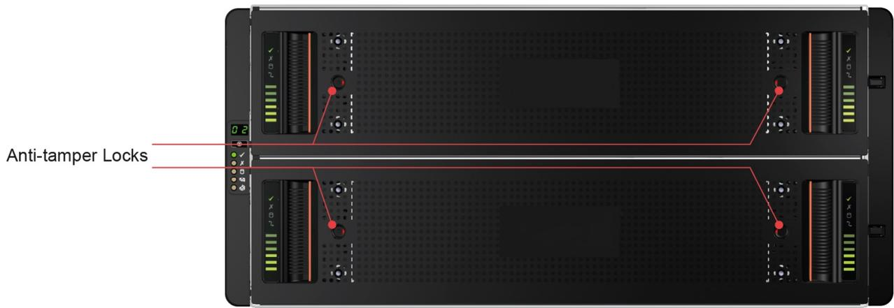
Figure 20. Verrous anti-effraction
