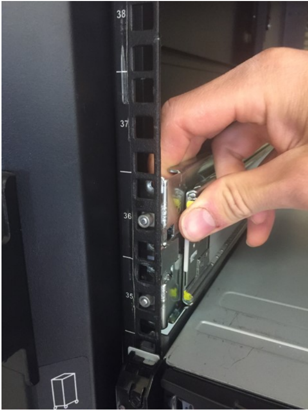
Figure 34. Front rack post attachment details
