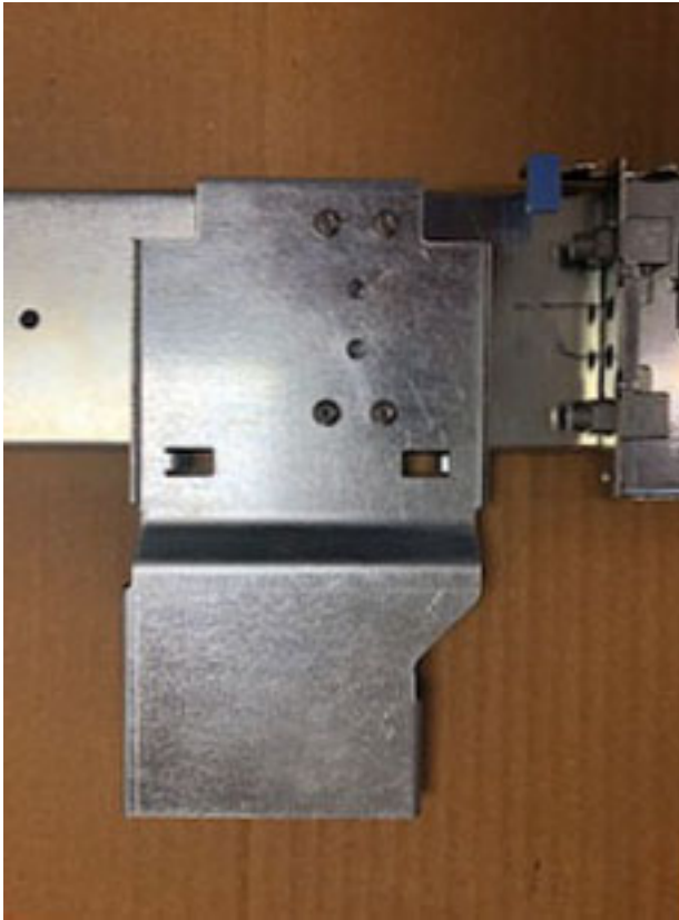
Figure 30. CMA attachment installed on outer slide
