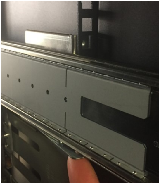
Figure 33. Attachment spring detail
