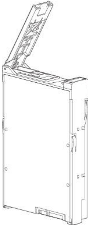
Figure 71. LFF drive carrier module in open position
