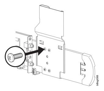
2. Attach 'C' bracket from rail kit to chassis with two screws (Item 1 under Table 1 on page 1) M4x4 PH. Torque: 12 lbf-in.
