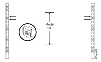
2. Use ten screws (Item 2 under Table 2 on page 1) to attach left and right rails to rack. Torque: 27 lbf-in.
