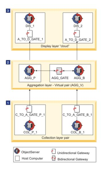
The diagram above depicts a standard three tier deployment with a Collection ObjectServer layer (1), an Aggregation ObjectServer layer (2) and a Display ObjectServer layer (3).
