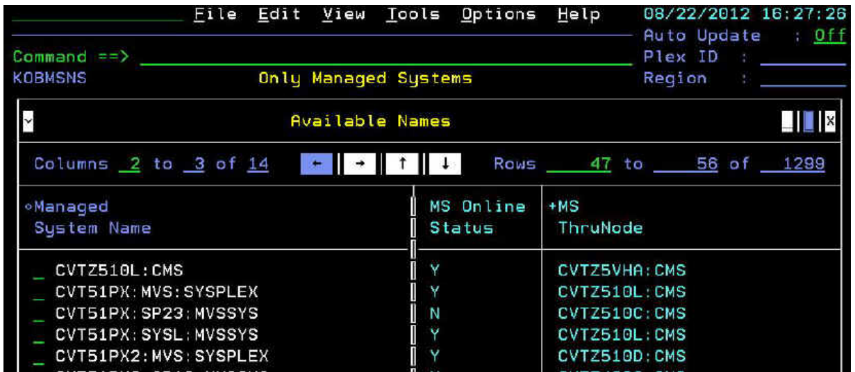
Figure 183. Only Managed Systems panel that lists the available names of the local registry.
