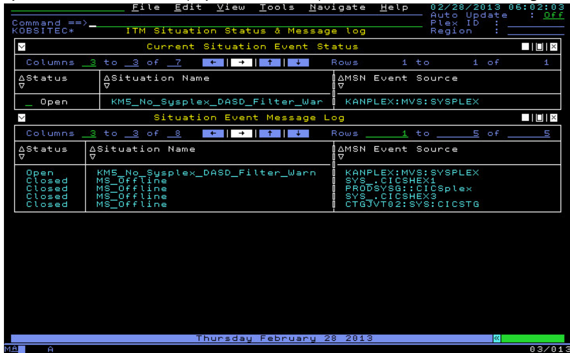
Figure 128. A cloned workspace is denoted by an asterisk (*) after the workspace name
