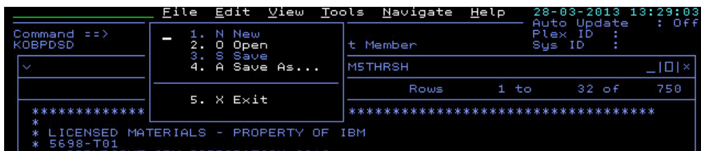
Figure 139. Cloning a threshold member by using the File > Save As menu option.
