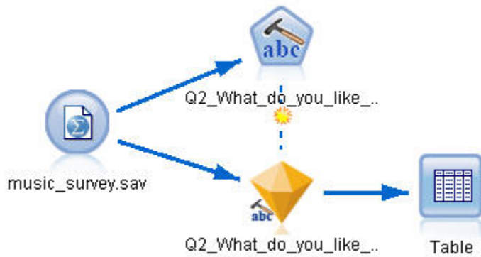
Figure 3. Example stream: Statistics File node with a Text Mining concept model nugget
