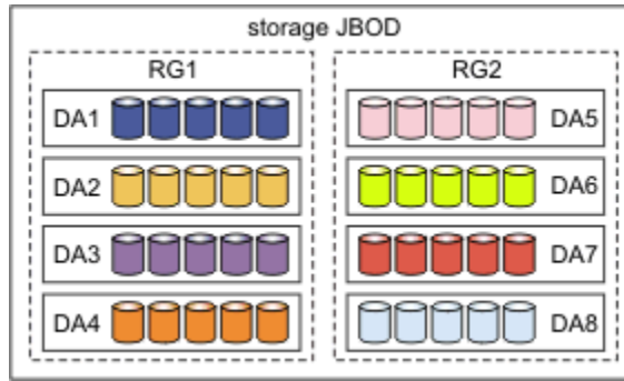
Figure 5. Example of declustered arrays and recovery groups in storage JBOD
