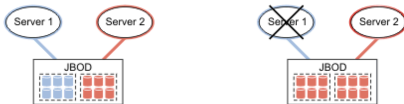
Figure 4. Minimal configuration of two IBM Spectrum Scale RAID servers and one storage JBOD
