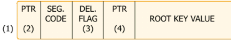
Figure 52. VSAM LRECL format as returned by buffer handler
