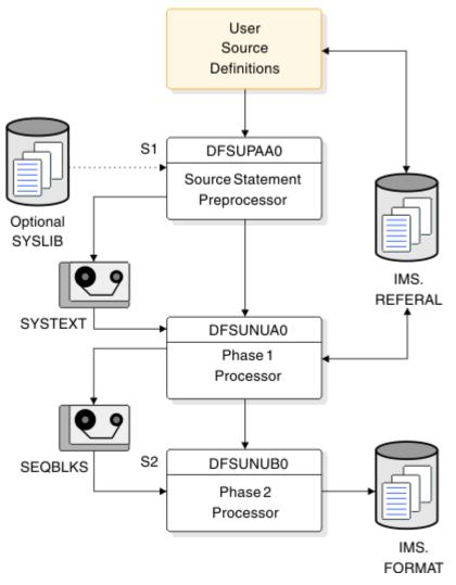
*Figure 8. Overall flow with the MFSUTL procedure*
