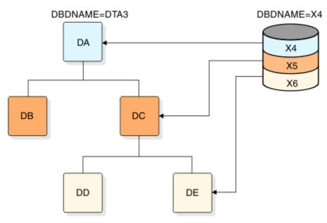
Figure 25. Database indexed by three secondary indexes in a shared secondary index database
