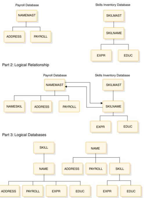
Figure 6. Logical relationship between physical databases and the resulting logical databases that can be defined
