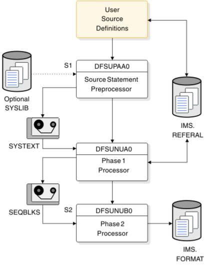
Figure 10. Overall flow with the MFSTEST procedure
