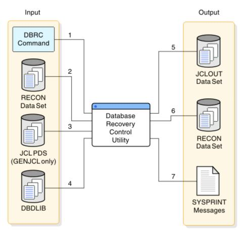
Figure 38. Database Recovery Control utility input and output
