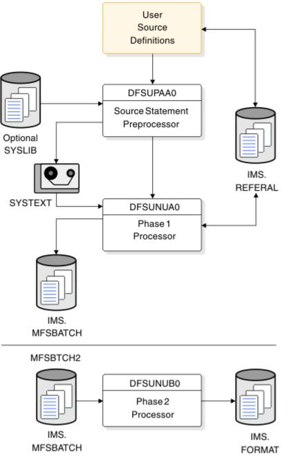
Figure 9. Overall flow with the MFSBTCH1 and MFSBTCH2 procedures
