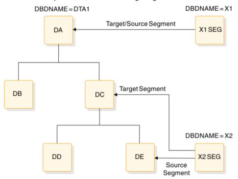
Figure 7. Database indexed by two secondary indexes
