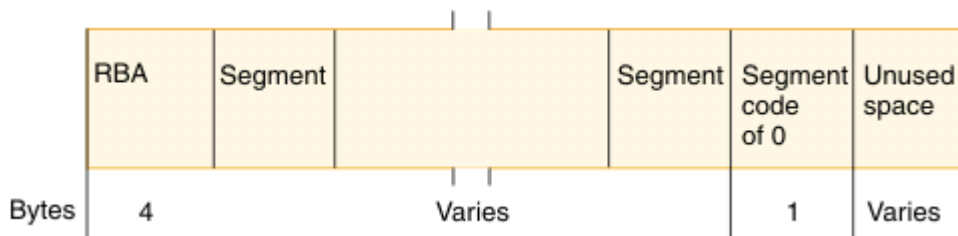
Figure 26. Format of a logical record in a HISAM database
