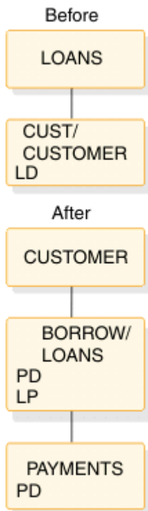
Figure 141. Logical child, virtual pairing—physical delete rule example: before and after
