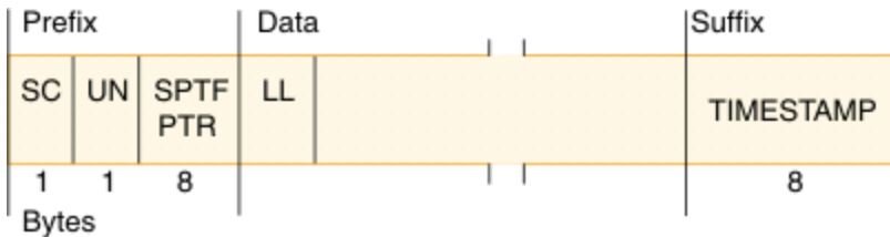
Figure 62. Sequential dependent segment format
