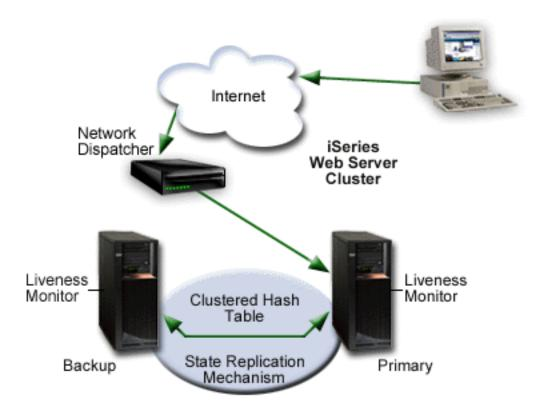
When the primary node fails (failover), or a switchover takes place, the failover/switchover process begins. The following steps are performed during failover/switchover:
