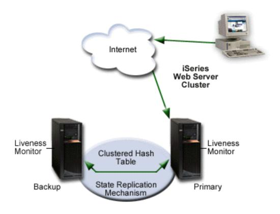
When the primary node fails (failover), or is brought down by the administrator, the failover/switchover process begins. The following steps are performed during failover/switchover:
